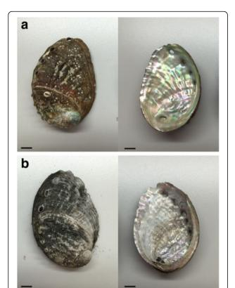
**Fig. 1** The SJM before (**a**) and after (**b**) calcined. SJM was placed in a metal pot and calcined, note the surface gloss was altered after calcined. Scale = 1 cm
